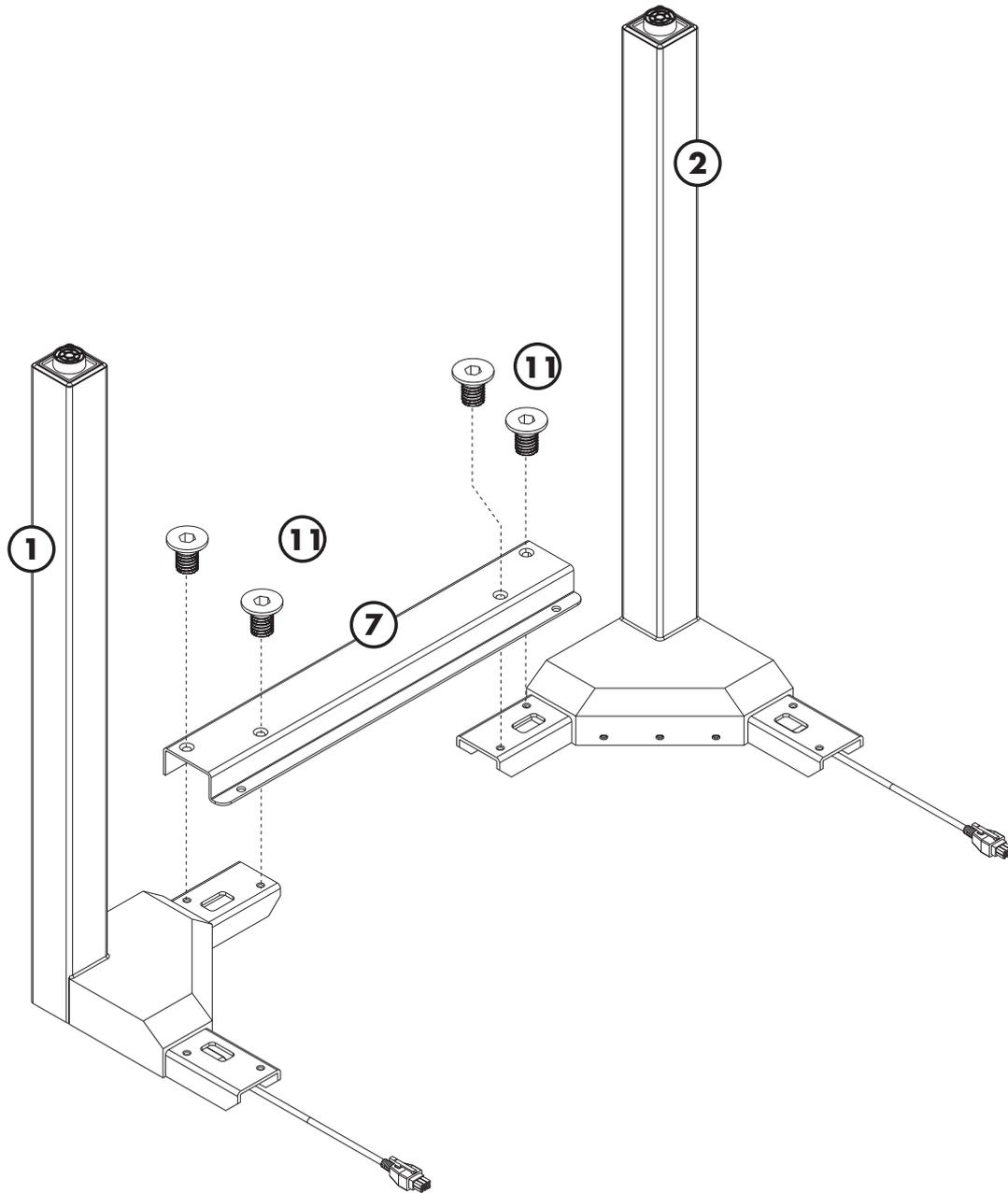
The table width can be extended with the help of 200 mm long spacers.
