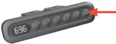
2. Following indication appears in the display, keep on holding the key
