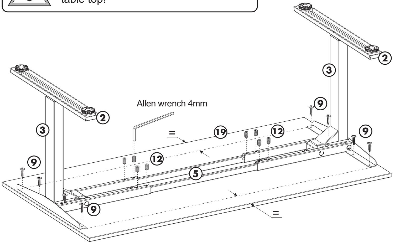
The frame of the desk is individually telescopic in width, in the dimensions 1200-1800mm. Therefore this frame is suitable for table top dimensions of:
