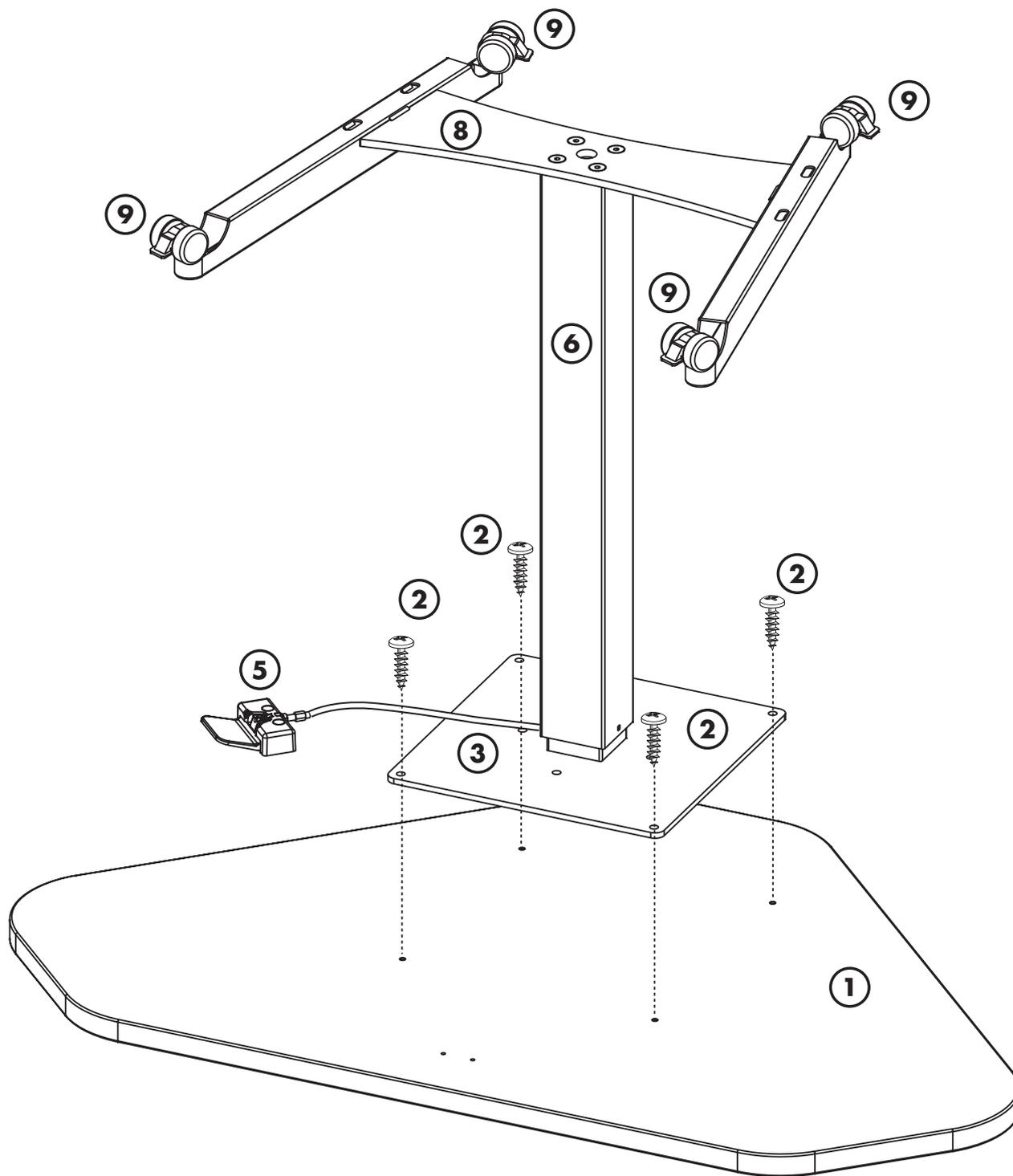
Use the fixing points on the underside of the desk top (holes with expansion sleeves) for mounting the panel to the frame.
