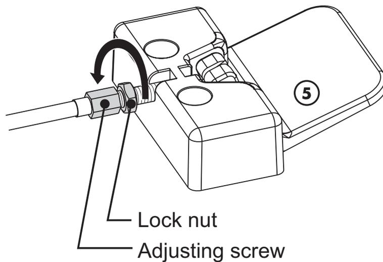
After adjustment, tighten the lock nut firmly.
