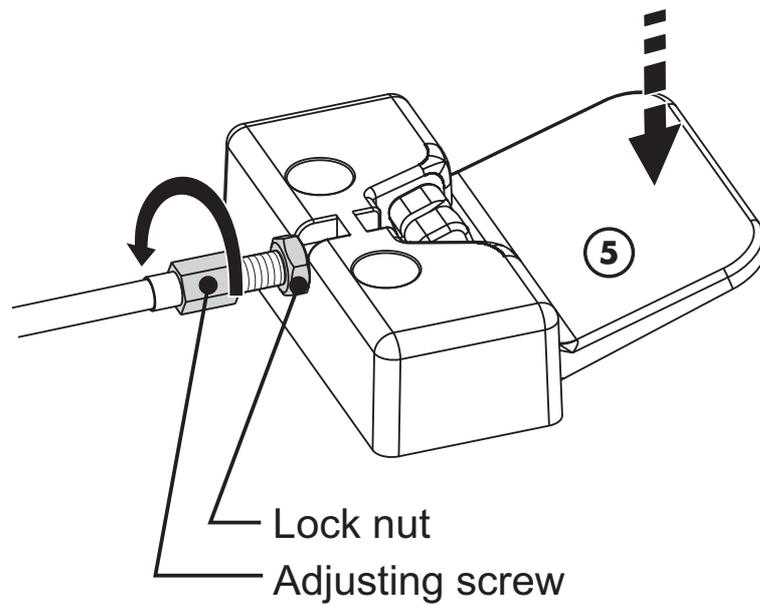
Turn the adjusting screw anticlockwise until the Bowden cable is under tension and the gas spring is released by pressing the actuator. Turning clockwise causes the gas spring to release less sensitively.
